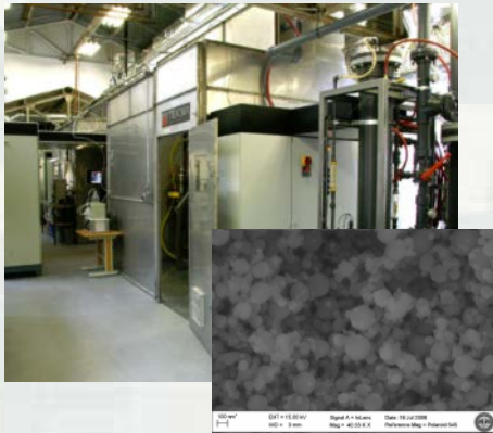
Tekna plasma system for nanoscale Al (above); SEM of nanoscale aluminum (below), Chris Haines, ARDEC
