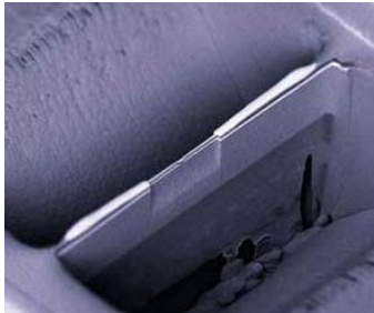
Sample preparation with FIB
