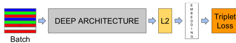
Figure 2. Model structure. Our network consists of a batch input layer and a deep CNN followed by L_2 normalization, which results in the face embedding. This is followed by the triplet loss during training.
